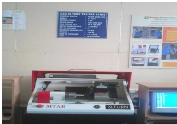
Fig. 1. Experimental set up using XLTURN- CNC lathe
